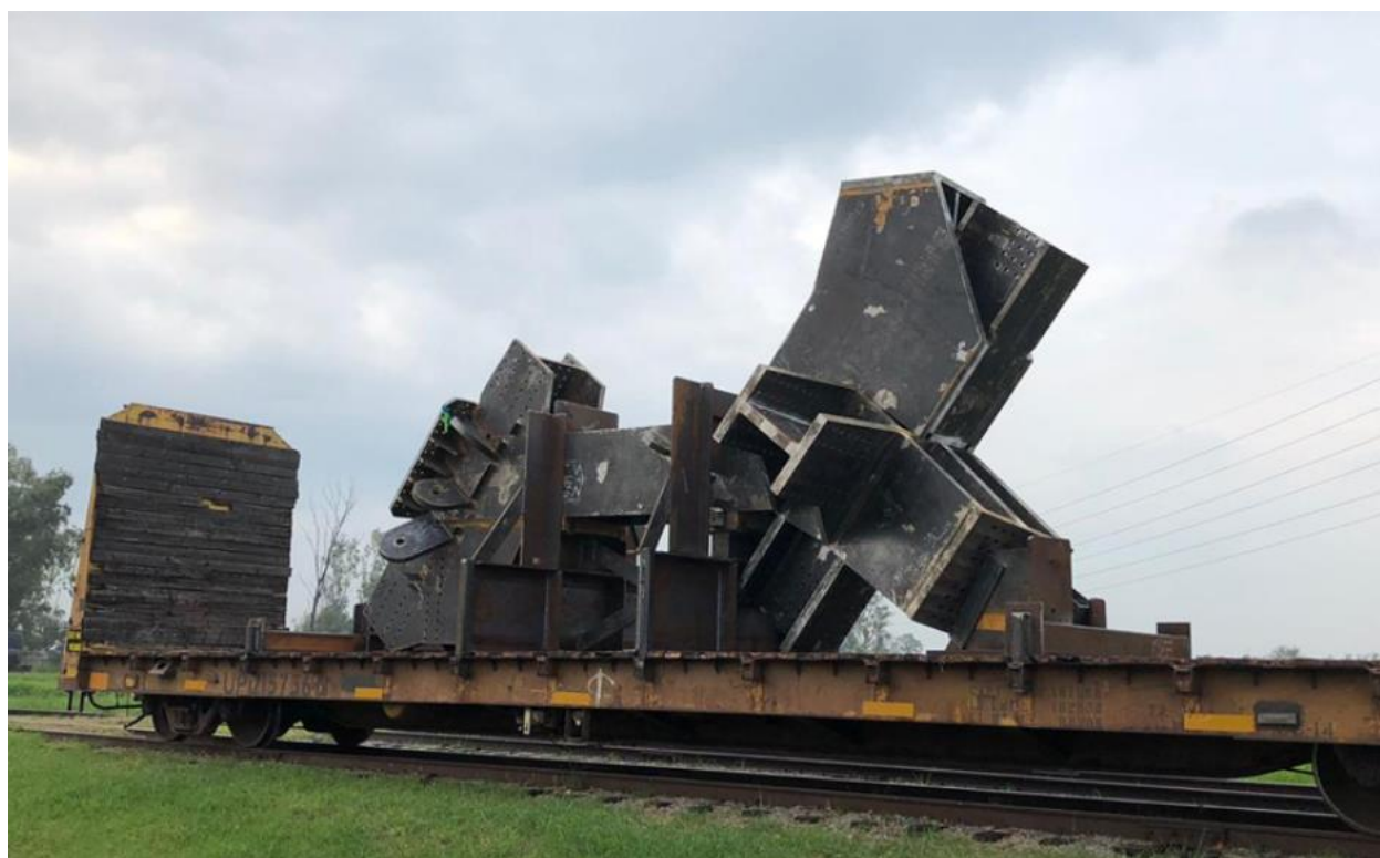
Figure 4-6. Steel connection – Two Manhattan West tower [48].
